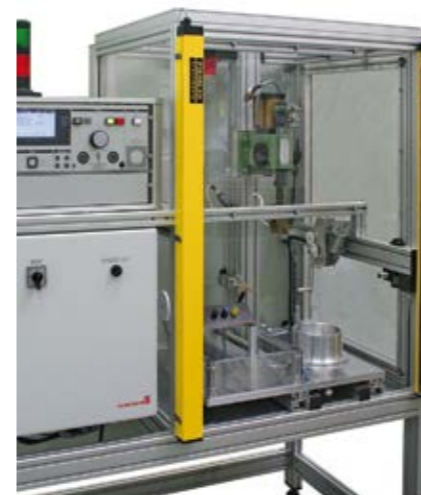
Test cover with light curtain in a customized solution
