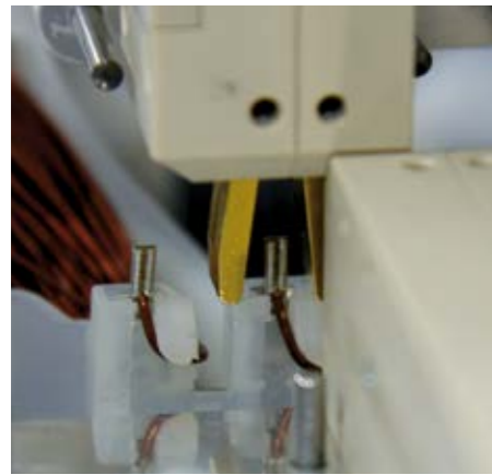
Contacting contact pins with Kelvin clamps
