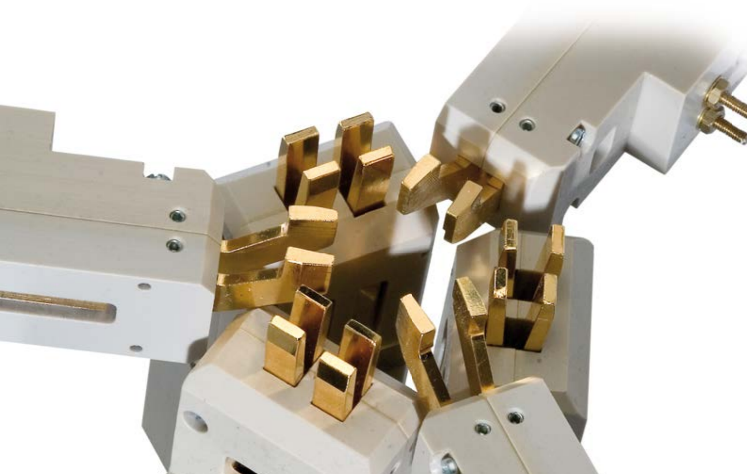
Contacting contact pins with Kelvin clamps
