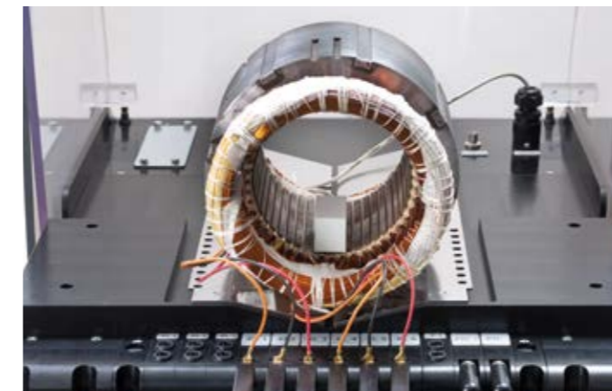
Loose rotary-field probe to be placed in the stator
