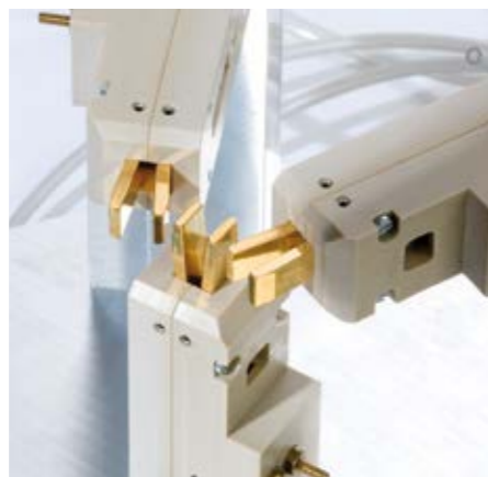
Contacting with pneumatic Kelvin clamps
