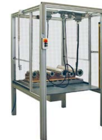
Large test cage with roller belt, light curtain and pneumatically controlled side doors
