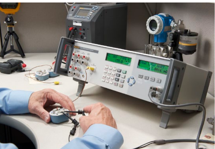
Thermocouple transmitter calibration
