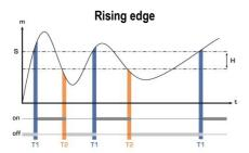
Measurement (m) > Threshold (S) during the time-delay  $T1 \rightarrow Alarm$
