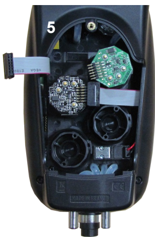
5 Insertion of a new sensor then rotation of the sensor
