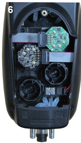
6 Connection of the sensor ribbon cable
