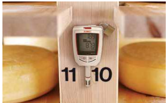
Relative humidity and temperature control in a maturing cellar using a KH 220 mounted onto a plate and secured with a padlock as part of a mapping process
