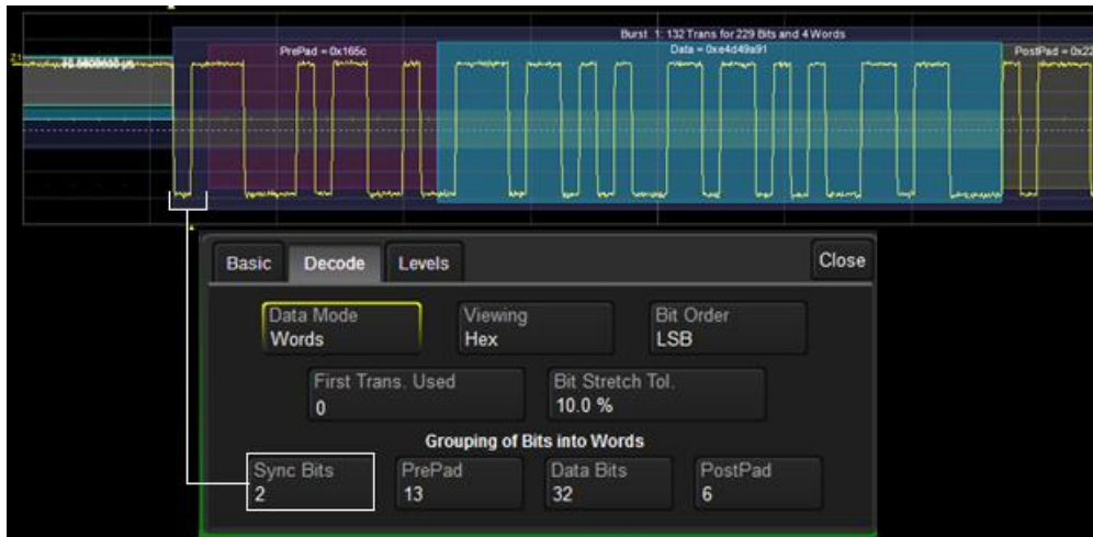
Figure 10: This zoomed segment shows one of four words in an NRZ signal. As specified in the Grouping of Bits into Words section of the corresponding Decode tab shown below the waveform itself, the word comprises 2 sync bits (bracketed in white), 13 PrePad bits, 32 data bits, and 6 PostPad bits
