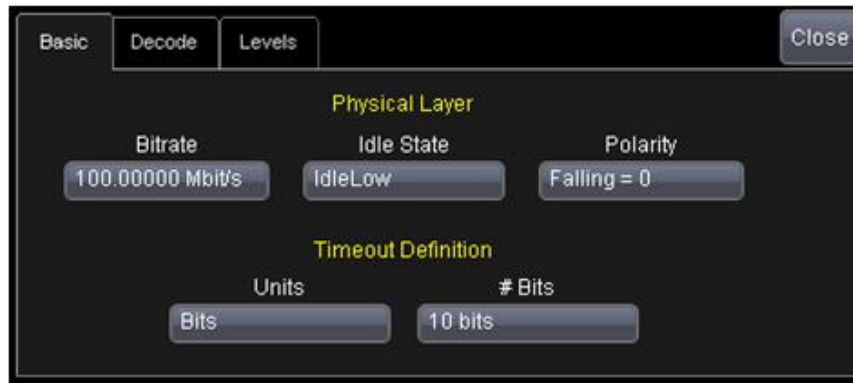
Figure 5: The three tabs (Basic, Decode, and Levels) driving Manchester bus decode
