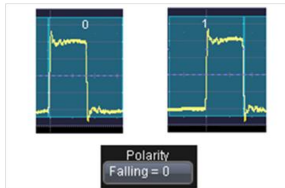
Figure 6: Manchester physical-to-logical mapping, case: Falling = 0
