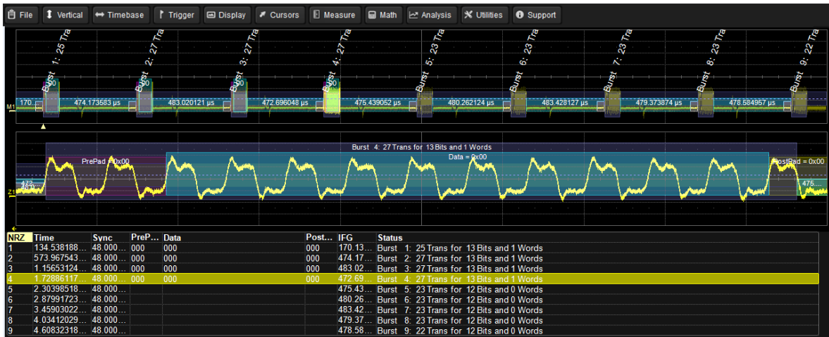
Figure 12: An interactive, configurable data table provides details about each data burst in the waveform
