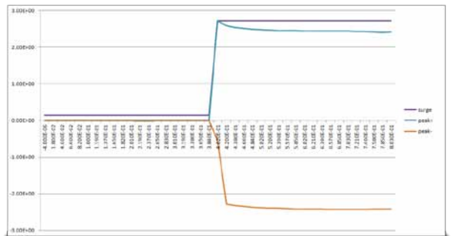
Example Inrush current data, datalogging at nominally 20ms intervals directly to PPALoG
